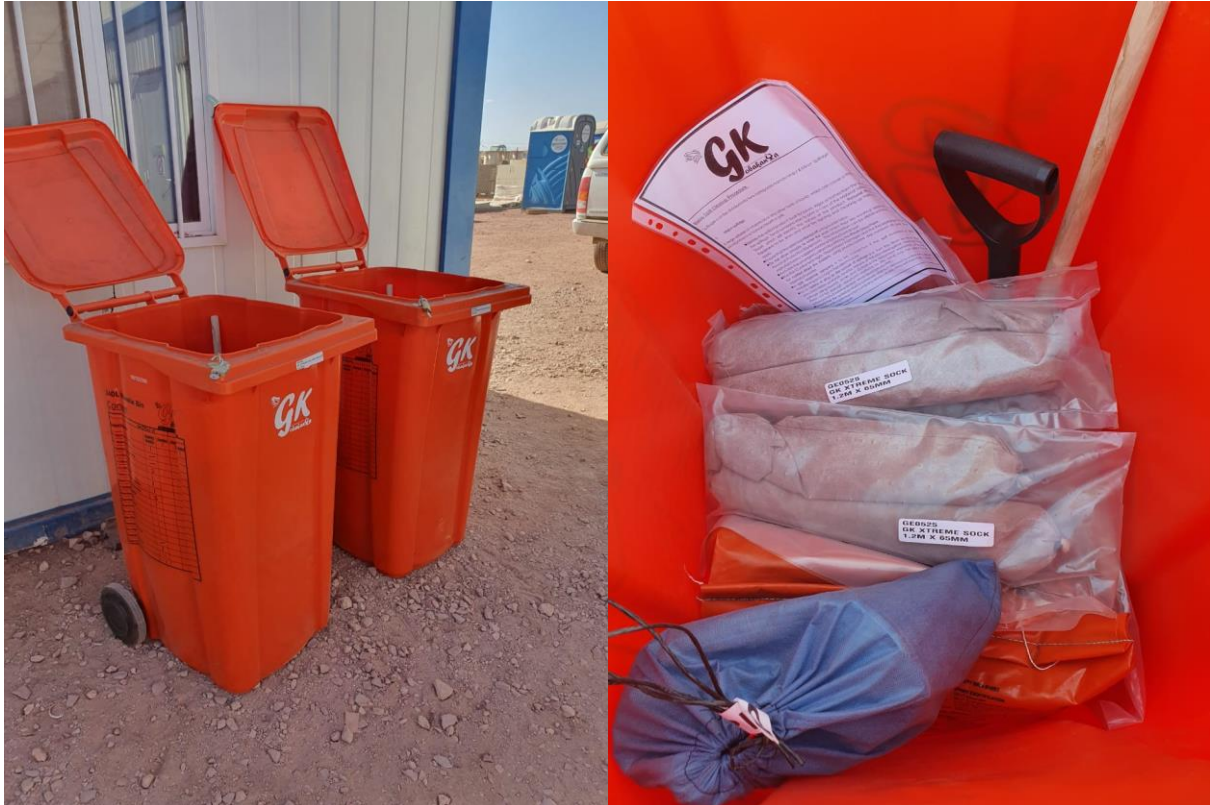
Figure 15: Hydrocarbon Spill Kits must be in place within the site camp and in the field within 500m of any drilling or ramming activity.
