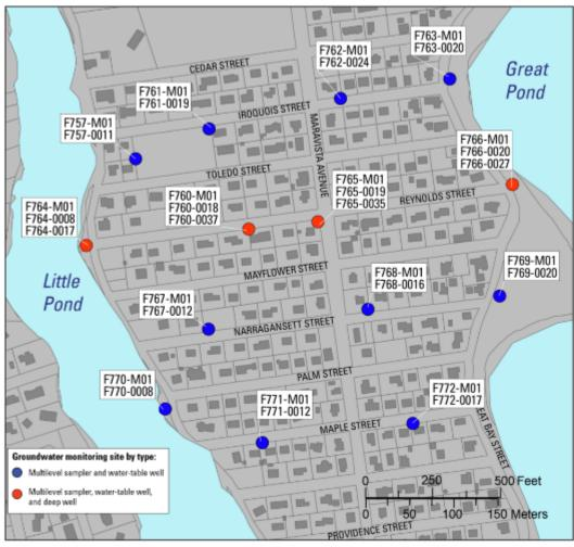
"F" in site name shorthand for MA-FSW; "M01" in site name indicates 15-port multilevel sampler; For monitoring wells, four digit number after site name reflects depth of well below land surface, in feet (e.g. MA-FSW 764-0017)
