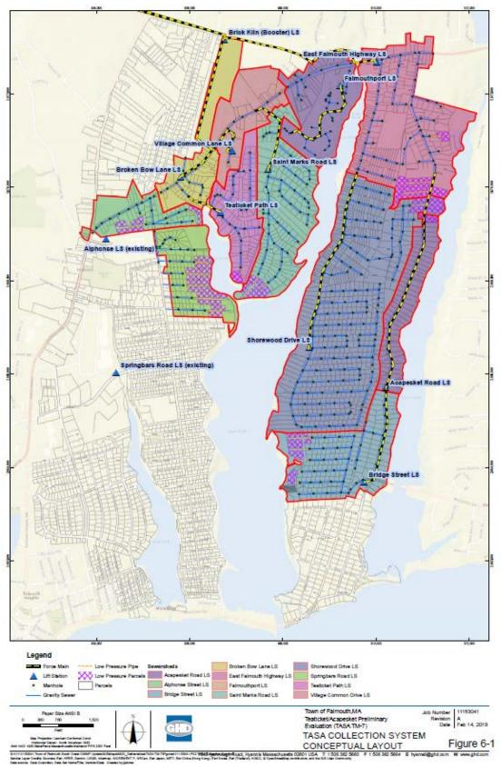
Figure 6.1 TASSA Collection System Conceptual Layout
