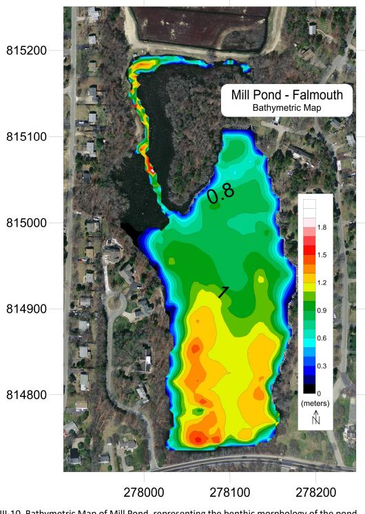
Figure III-10. Bathymetric Map of Mill Pond, representing the benthic morphology of the pond.Report- CSP/SMAST:FALMOUTH, Mill Pond Assessment
