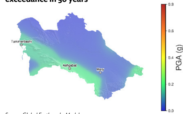
Figure 18: Seismic hazard map for peak ground acceleration (PGA) with a 10% probability of exceedance in 50 years
