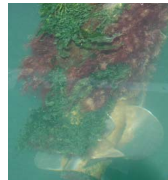
A heavily fouled propeller of a recreational boat that may transport organisms from one location to another. Photo credit: J. Pederson
