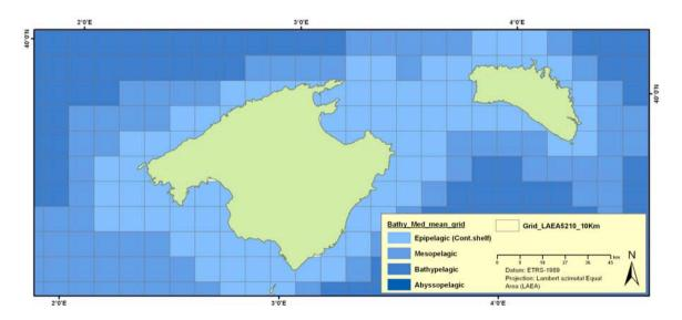
*Figure 12.* The resulting layer after the assignation of an averaged value for each 10 km cell. A further classification was performed using a new field (Pelagichab).
