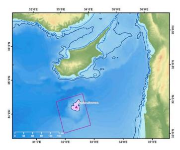
**Figure 20.** Using the bathymetric contours the 1.000 m depth contour enclosing the peak is selected and converted into a polygon for each of the seamount. A seamount can be defined as steep-sided feature, rising 1.000 m or more from the sea floor and not tall enough to break to the sea surface and turn into islands. In the Eratosthenes example, the FRA boundaries enclosing the protected area are shown (Recommendation GFCM/2006/3).
