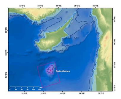
*Figure 21.* Using the bathymetric contours a seamount is defined by the 1.000 m depth contour enclosing the peak. This contour is converted into a polygon for each of the features. In the Eratosthenes example, the FRA boundaries enclosing the protected area are shown (Recommendation GFCM/2006/3).
