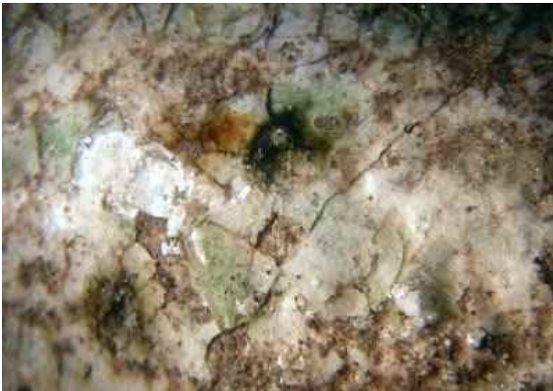
Fig. 31. Detail from Fig. 14 in close-up. The colourless to greenish glass exhibits many minute vesicles. The field is 22 mm wide.
