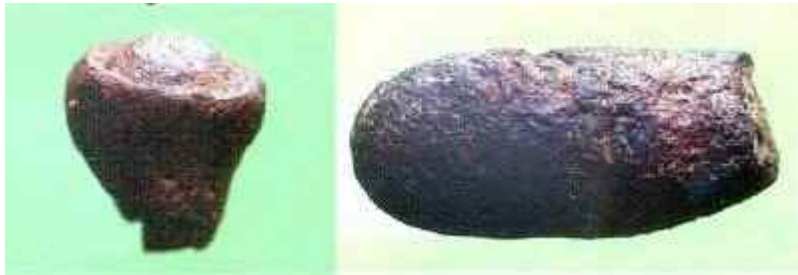
Fig 37. "Splash" shapes indicating rapid cooling and solidification of glass particles during flight.
