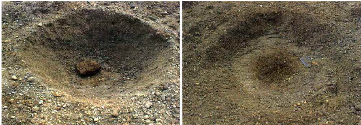
Fig. 15. Uncovered secondary cratering. Projectile (to the left) and halo of discolored host rock.
