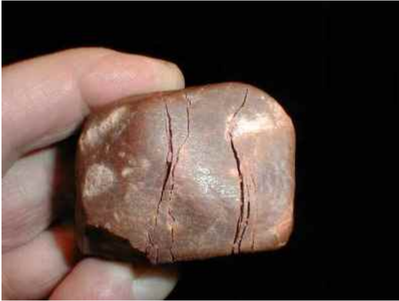
Fig. 27. Spallation fractures in naturally shocked quartzite cobble. Buntsandstein conglomerate near Rubielos de la Cérída impact basin.
