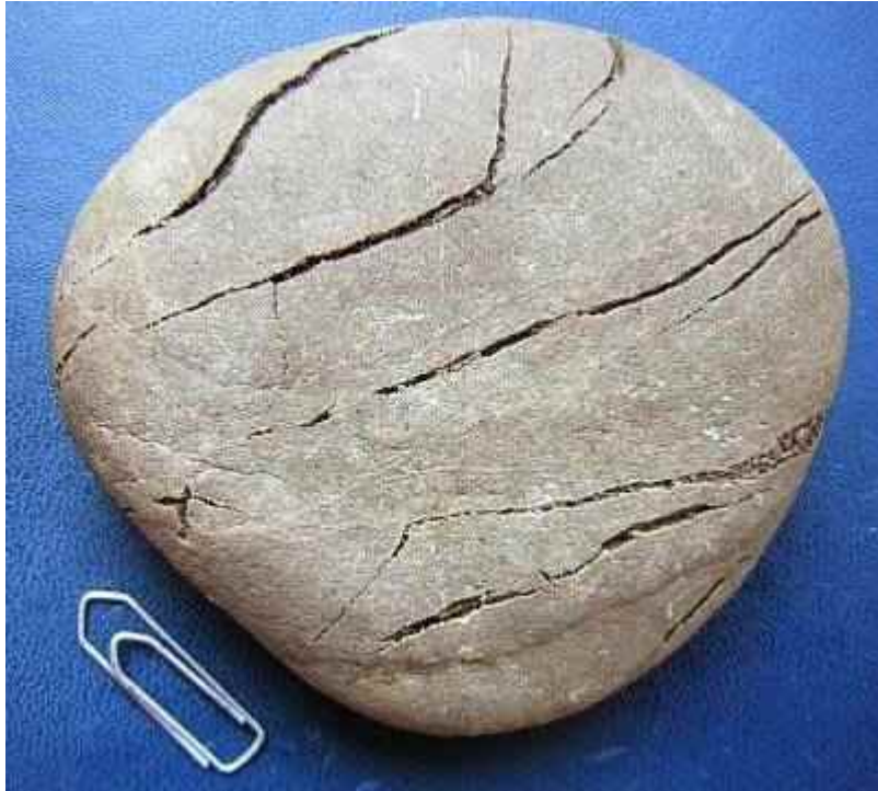
Fig. 25. Spallation fractures in a sandstone cobble from crater 016 in the Chiemgau strewnfield.
