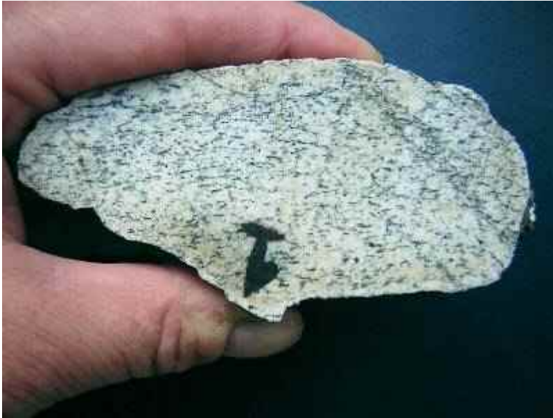
Fig. 32. Sawed surface of a thermally shocked sandstone cobble completely coated by silica glass. Note the dark strings of partly recrystallized feldspar glass giving a gneiss-like aspect to the rock. From 11 m-diameter crater 004.
