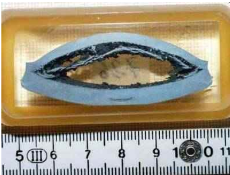
Fig. 26. Spallation fractures in experimentally shocked ARMCO iron (by courtesy of M. Hittl).
