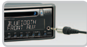
Front auxiliary input for connection of portable audio player or other equipment
