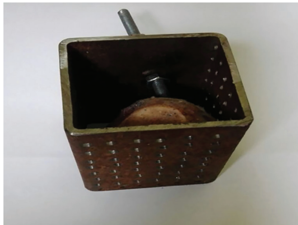
Figure 6 - Side view of a device for bone allograft channeling with subsequent impregnation of drugs into the bone tissue with femoral bone head fixed in it
