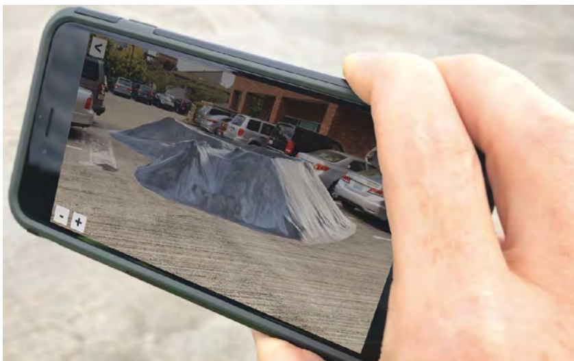
Stockpile Reports Lite, a new app available on the latest iPhone, enables the user to project a 3-D stockpile wherever the phone is pointed. Above, a virtual stockpile is dropped on a parking lot. (Photo: Stockpile Reports)
