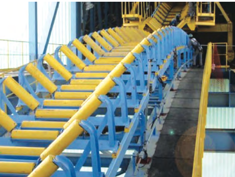
Metso says its Energy Saving Idler system reduces the load typically carried by conventional roller systems by 50%, in addition to cutting belt power consumption by up to 35%.
