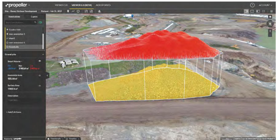
The Propeller Site Intelligence Platform features tools that facilitate determination of volumetrics, run-of-mine values, pit volumes and monthly reconciliations. (Image: Propeller Aero)
