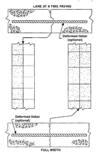
Fig. 4.5—Longitudinal joints.<sup>33</sup> (Note: use butt joint with tie bar for pavements 150 mm [6 in.] thick or less.)
