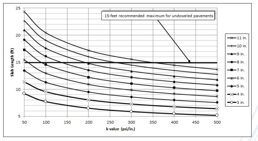
Using the criterion of a maximum L/ $\ell$  ratio of 5.25, the allowable joint spacing would increase with increased slab thickness but decrease with increased (stiffer) foundation support conditions.
