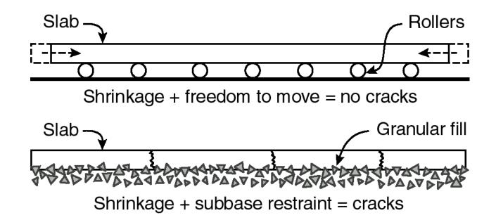
Shrinkage + Restraint = Cracking
