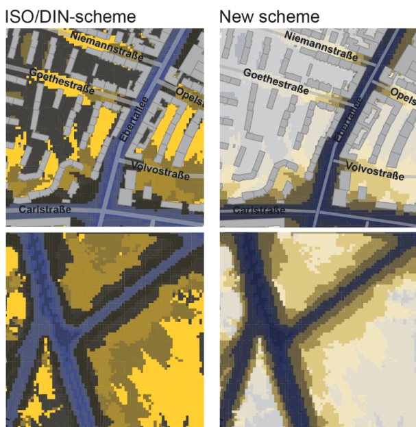
Figure 4: Fig. 3 simulated for color vision deficiencies (deuteranopia). With the ISO/DIN scheme the class 40-45 dB can be mistaken for the classes 60-70 db. (Simulated with the software eye.syde .)
