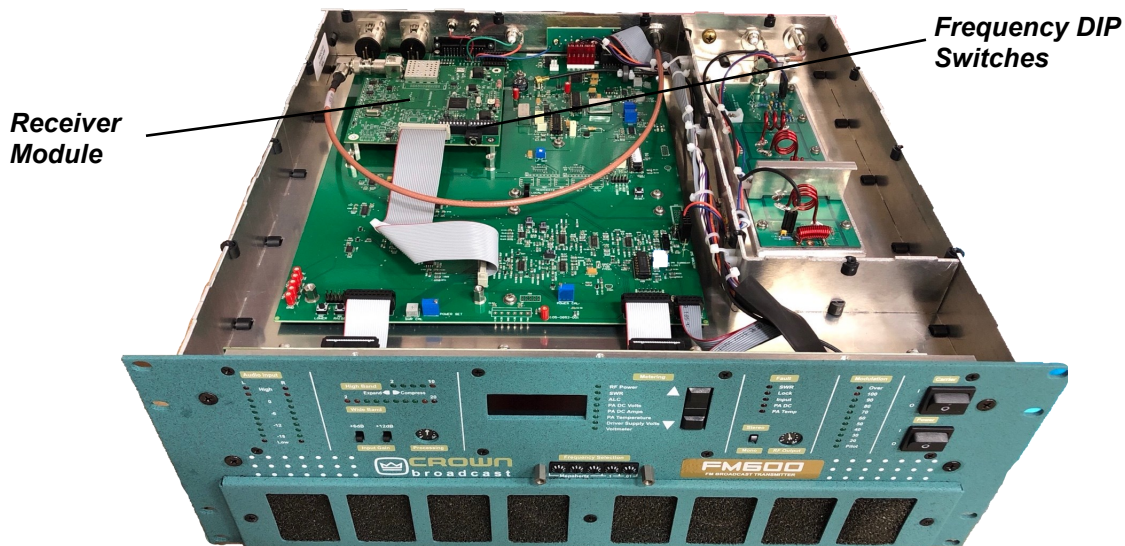
Illustration 2-11 CHT-1 Receiver Module Frequency DIP Switches
