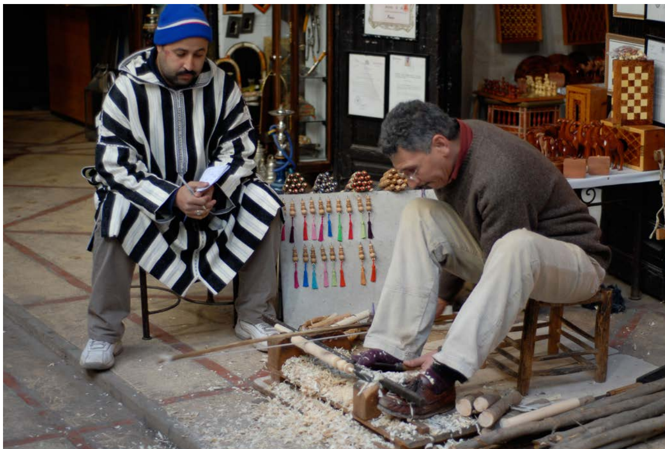
Figure 24.7 A craftsmen in Morocco working with a bow lathe (photo: Alamy stock photos).
