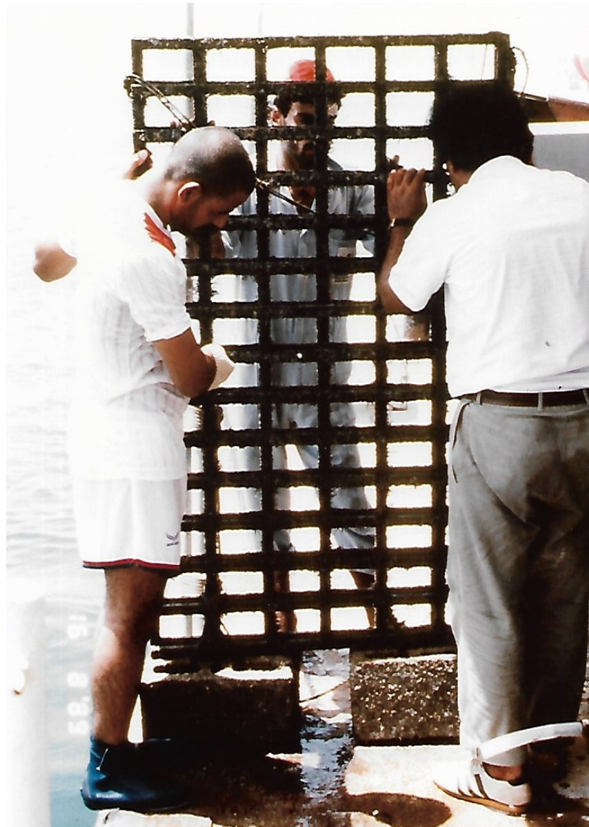
Wooden frame coated with bitumen
