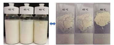
Fig. 3: The sample vials (left) and their quality control test (right) at the end of the measurement at 42  $^\circ$ C, 45  $^\circ$ C and 48  $^\circ$ C, respectively.
