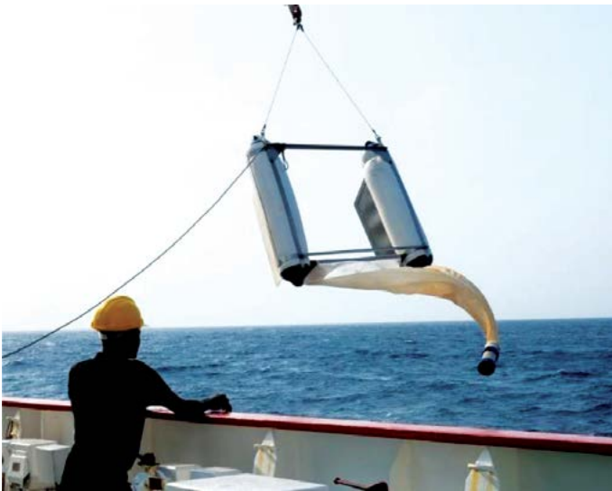
Figure 1: Neuston net deployment off the SA Agulhas II
