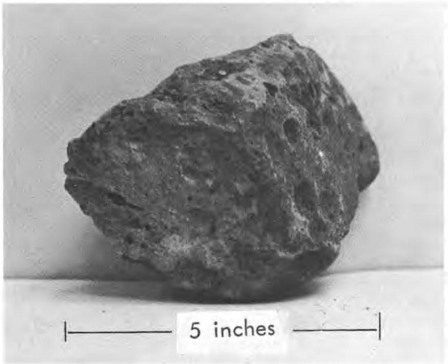
FIGURE 11.—Typical bauxite nodule that has weathered out of the ore zone. Note the pitted or vuggy appearance, which is also typical.
