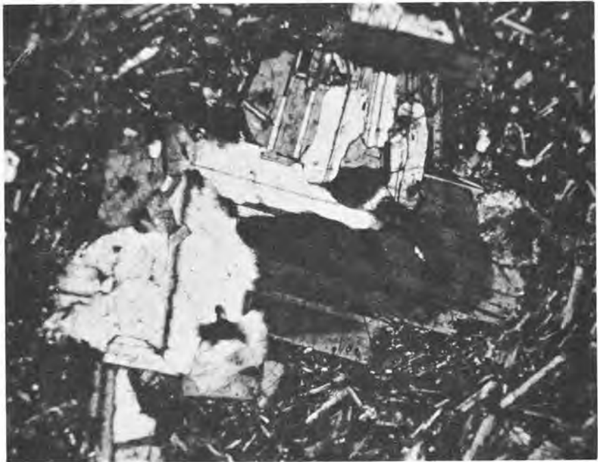
FIGURE 2. — Photomicrograph showing typical clots of plagioclase phenocrysts in volcanic flows of the Cowlitz Formation. This is also typical of Goble Volcanics. (X 50—crossed nicols.)
