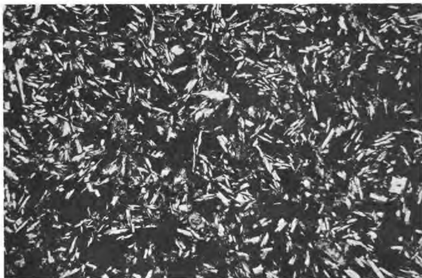
FIGURE 4.—Photomicrograph of Columbia River Basalt. White crystals are plagioclase and augite. Black area is volcanic glass heavily charged with an opaque mineral dust, probably magnetite. (X 18—plane light.)
