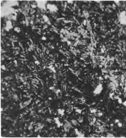
FIGURE 12.—Photomicrograph of bauxite nodule, using plane light, showing relict igneous texture. (X 50.)
