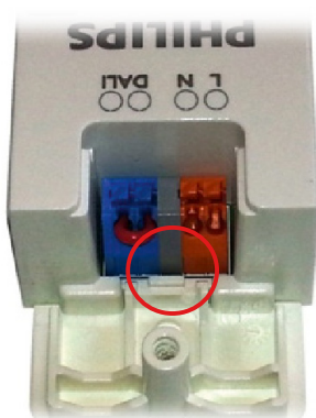
DALI driver used as fixed output
