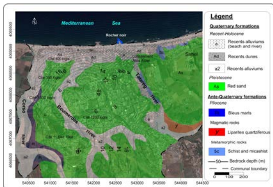
Figure 4 : Geotechnical and hydrogeological map Boumerdes site
