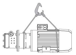
*Fig. 5-1 Transporting the pump with a crane*
