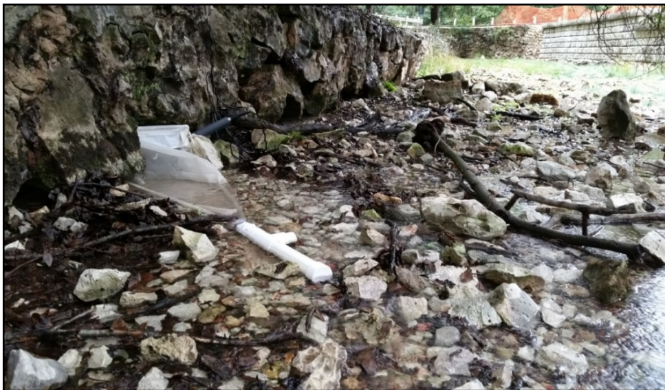
Drift net over Spring Run 1 orifice showing net placement and orientation to the spring.
