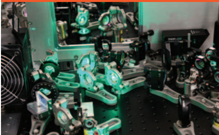
Cross-correlator: active timing jitter stabilization of pump (green) and signal (red) pulses
