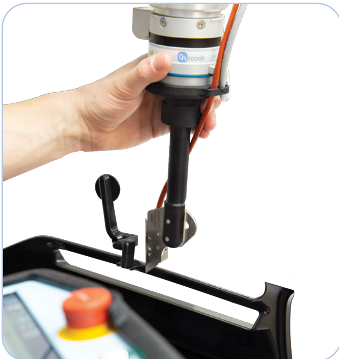
OnRobot HEX Force / Torque Sensor with Gimatic Hot Blade (Q#7286). Degrate by teaching your cobot the gate location, force required and part geometry.
