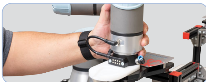
Teaching your cobot the home position is easy with the EOAT pickup position teaching tool. Contact EMI for more information.
