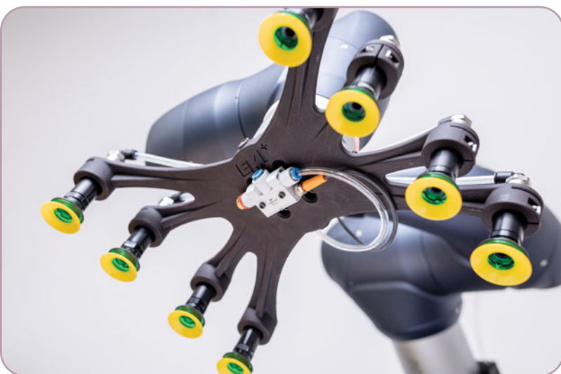
The lightweight 3D printed EOAT above can hold up to a 10k payload.
