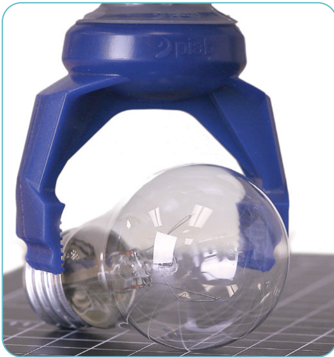
#8071 Two-finger gripper can grip sensitive and lightweight objects with odd geometries.
