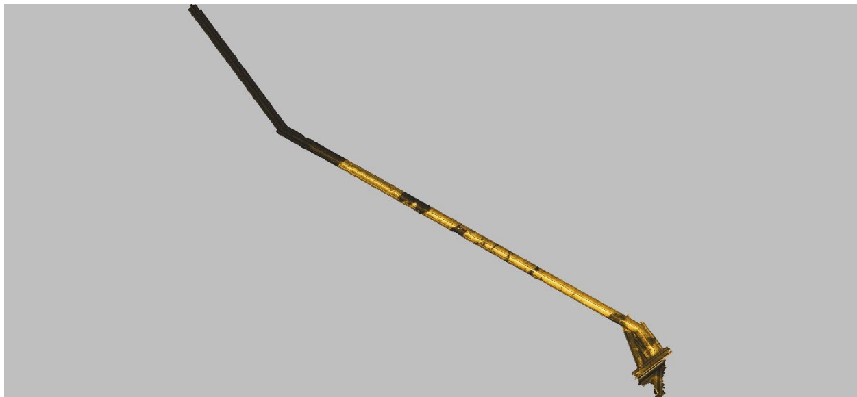
Figure 18. Side scan sonar mosaic of sediment type (dark brown= silt/clay, lt. brown =sand/gravel).
