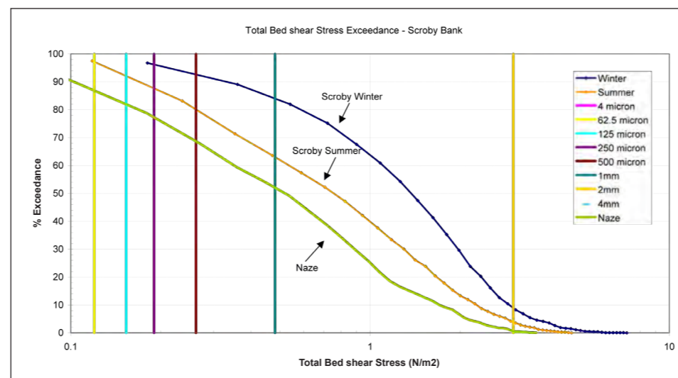
Figure 2.11 Bed shear stress exceedance diagram for Scroby Sands (Cefas, 2004) in 5 m water depth. The Naze Line is a monitoring point off Harwich used in SNSSTS 2.
