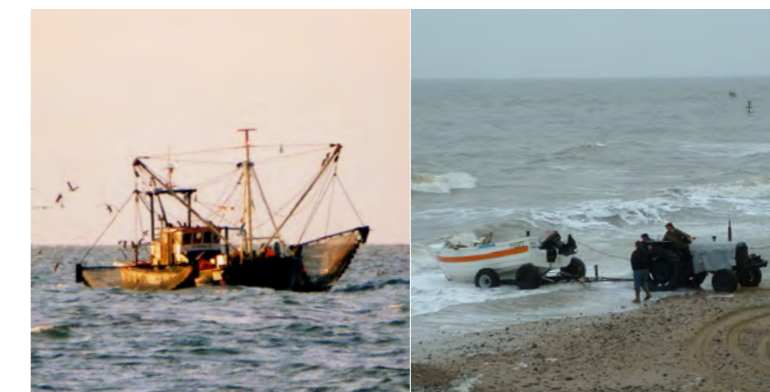
Figure 2.53 Types of fishing vessel used in the East Coast REC Study Area to catch crustaceans. Left: beam trawler catching brown shrimps; right: crab potter. © Crown Copyright 2011.
