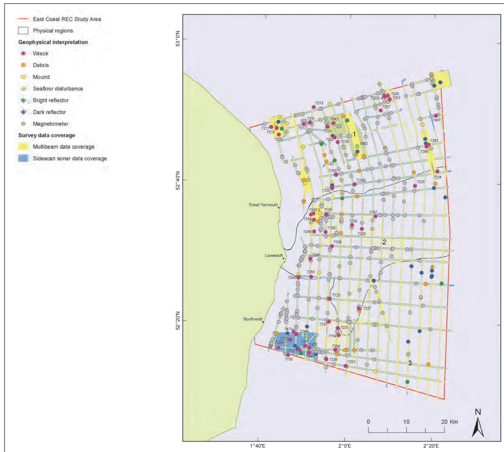
Figure 5.40 Distribution of geophysical anomalies in the East Coast REC Study Area.
