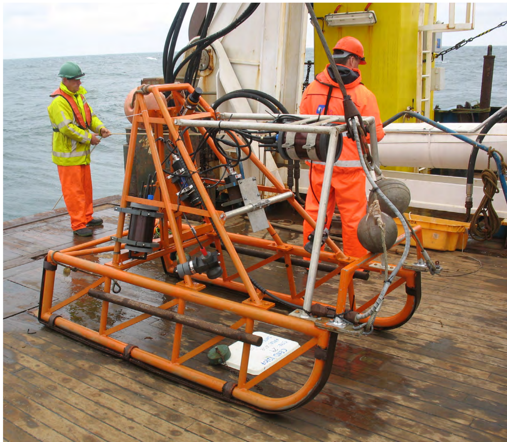
Figure 3.13 Conventional towed camera sled for collecting still and video images of the seabed. © Crown Copyright 2011.
