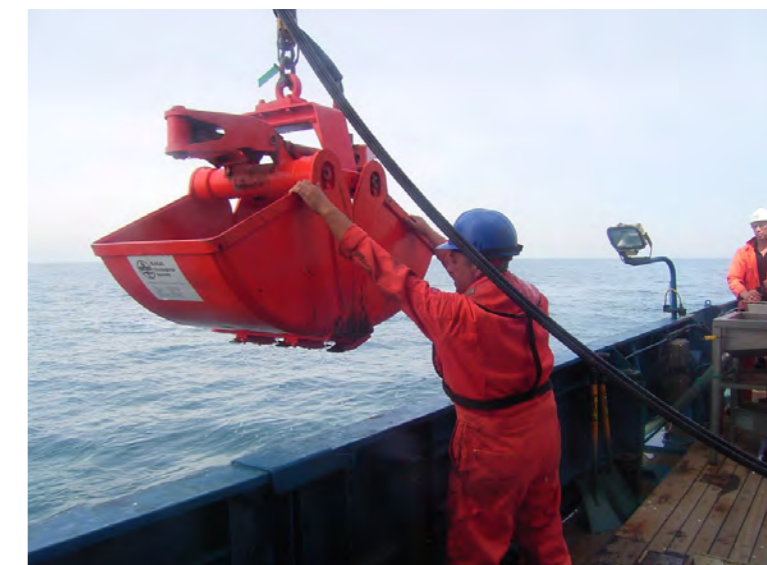
Figure 3.9 Hydraulically operated industrial “hopper-type” Clamshell grab with a 340 l capacity. © British Geological Survey.
