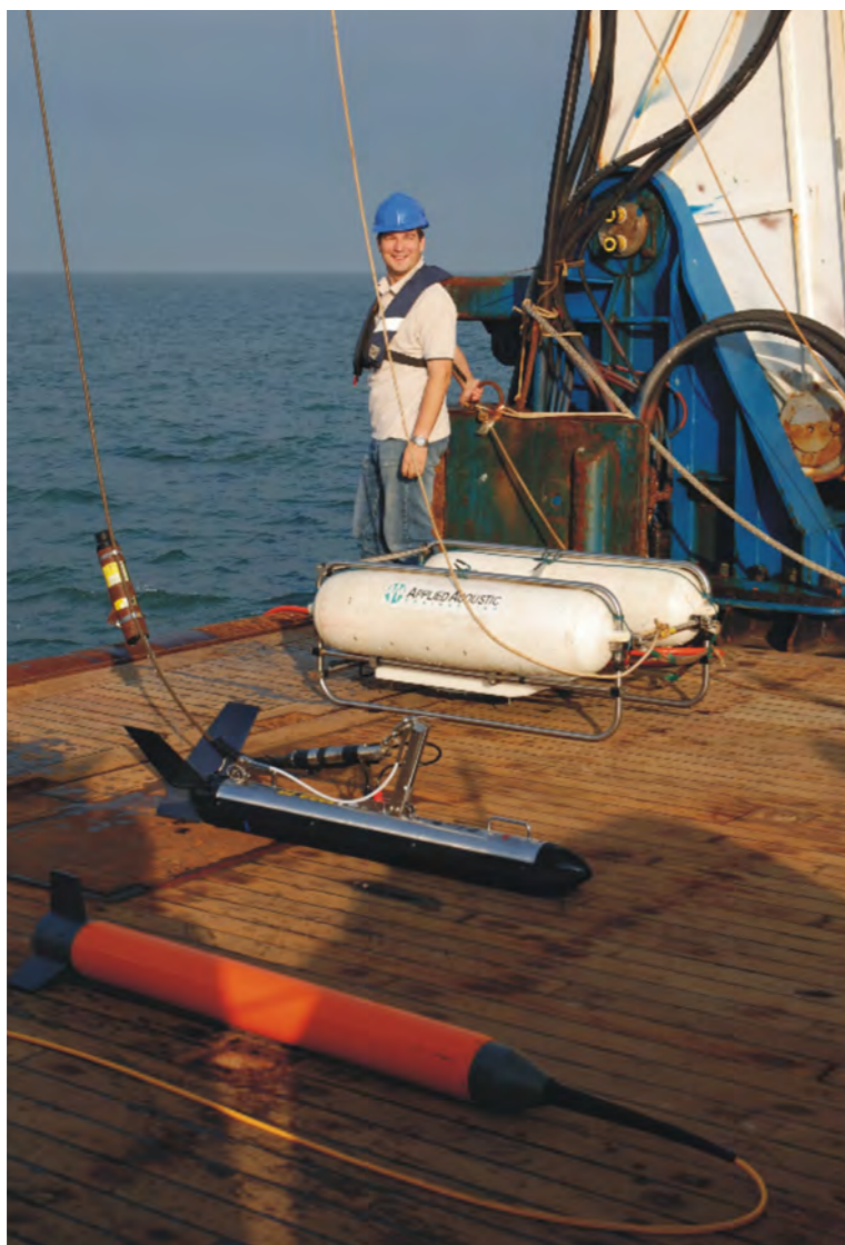
Figure 3.2 Boomer, side-scan sonar and magnetometer towed sensors (from front to back). © British Geological Survey.
