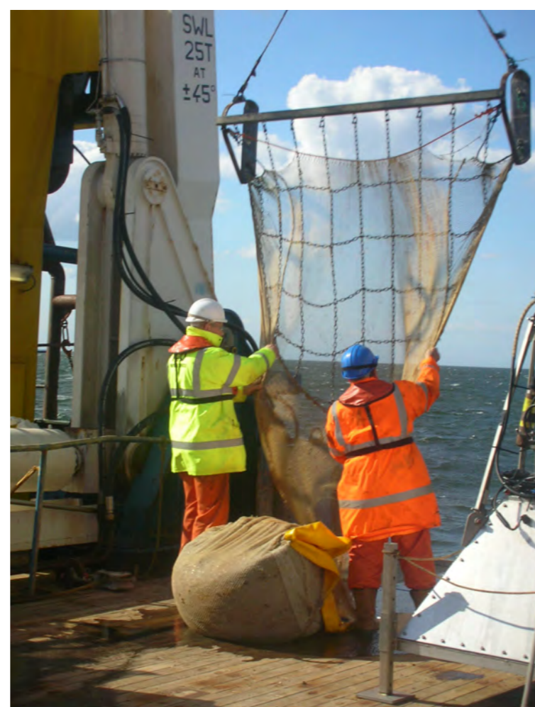
Figure 3.11 A Jennings 2 m scientific beam trawl with a chain mat and cod-end chafer. © Crown Copyright 2011.
