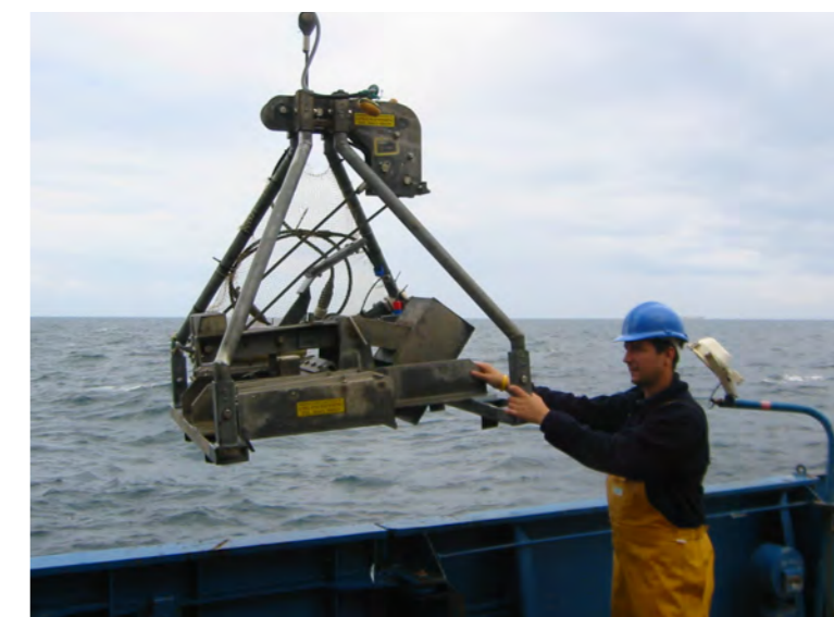
Figure 3.10 0.1 m 2 Hamon grab. © Crown Copyright 2011.
