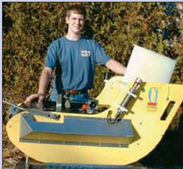
An undulating oceanographic recorder, towed behind a ship, is used to collect ecological parameters needed to assess the state of the marine ecosystem (Jerome Prezioso, NOAA NMFS).
