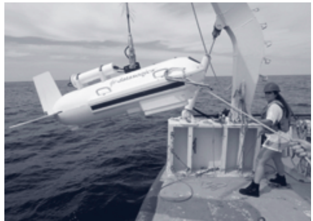
A sub-bottom profiler allows geologists to get data about the seafloor and the structure below. (photo: Dan Blackwood, USGS)
