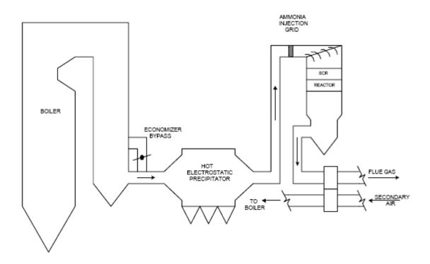
Figure 2.8: Low-Dust SCR Arrangement [46]
