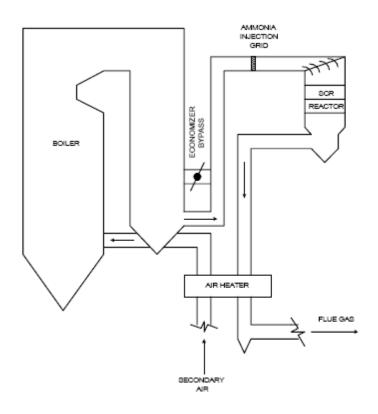
Figure 2.7: High-Dust SCR Arrangement [46]
