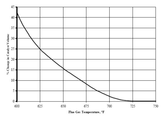
Figure 2.3: Change in Catalyst Volume vs. Temperature [56]
