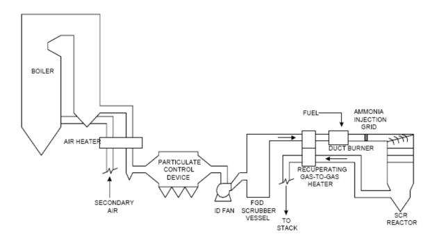
Figure 2.9: Tail-end SCR Arrangement [46]
