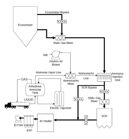
Figure 2.1: SCR Process Flow Diagram [35, 36]
