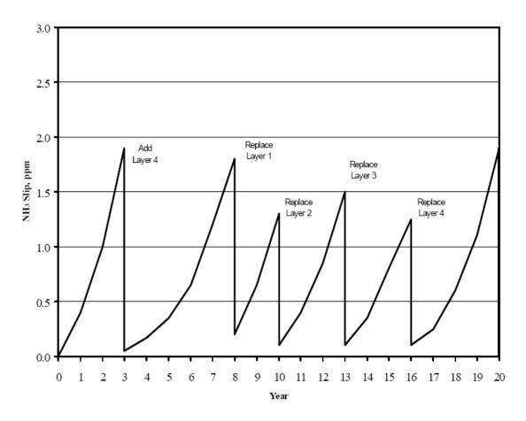
Figure 2.6: Typical Catalyst Management Plan [71]
