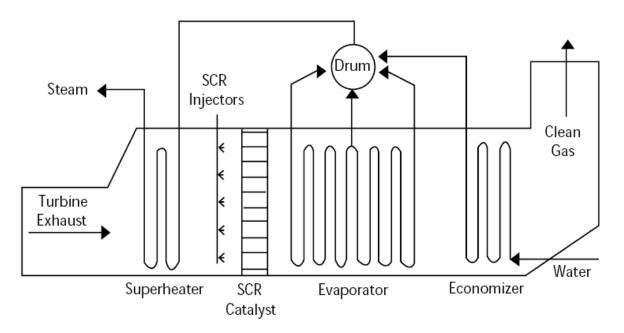
Figure 2.10: SCR Arrangement for a Combined-Cycle Gas Turbine [46]
