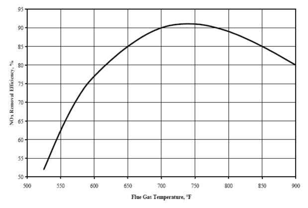
Figure 2.2: NO<sub>x</sub> Removal versus Temperature [50]
