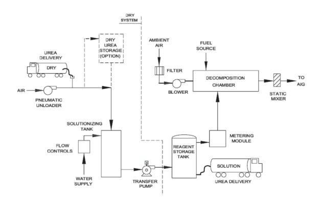
Figure 2.12: Urea-Derived Ammonia Production System Using NO<sub>x</sub> ULTRA System [87] Used by permission of K.R. Dougherty of Fuel Tech, Inc.
