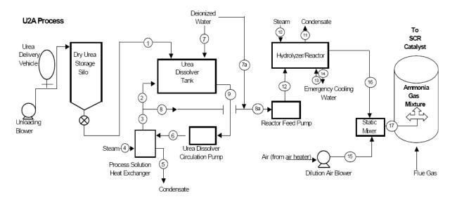
Figure 2-11: Urea-Derived Ammonia Production System Using U2A system [84] Used by permission of R. Salib of URS Washington Division (formerly Washington Group International).
