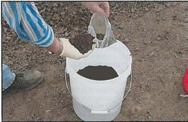
Figure 3. Place solid manure samples in a resealable freezer bag.
