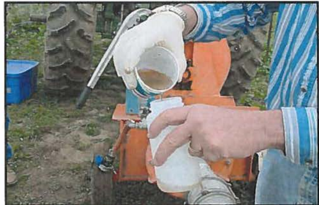
Figure 7. Put liquid manure samples in plastic, screw-topped containers.
