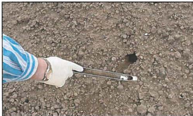
Figure 1. A soil probe can help provide a representative sample.
