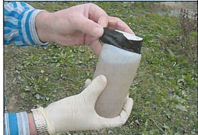
Figure 8. Seal liquid manure samples carefully.
