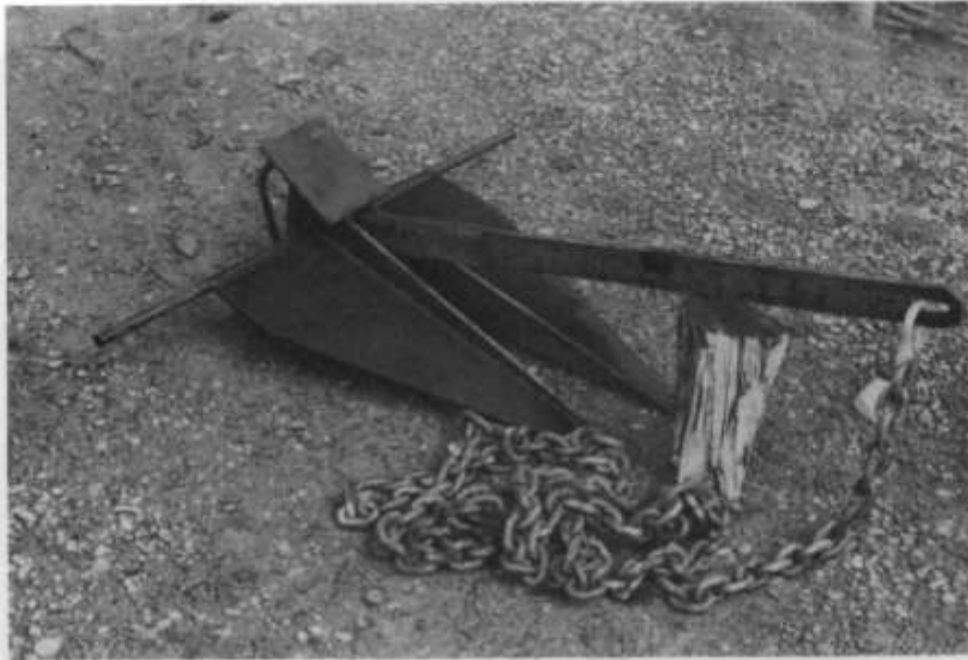
Fig. 60. Several types of plate-plow anchors (approx 50kg) used for mooring long lines or rafts.
