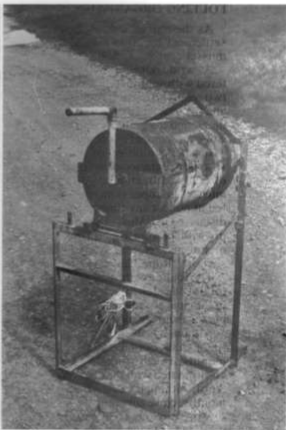
Fig. 40. (Above Right) Hand powered declumping apparatus. (Below) Close up of centre revolving shaft and pegs and adjustable cross chains.
