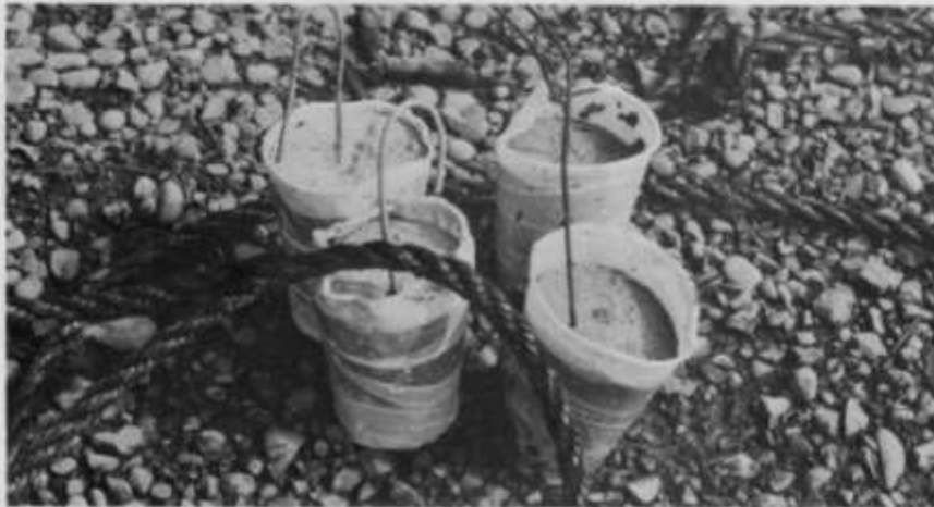
Fig. 64. Rope weights are usually poured in 600ml milkshake containers.
