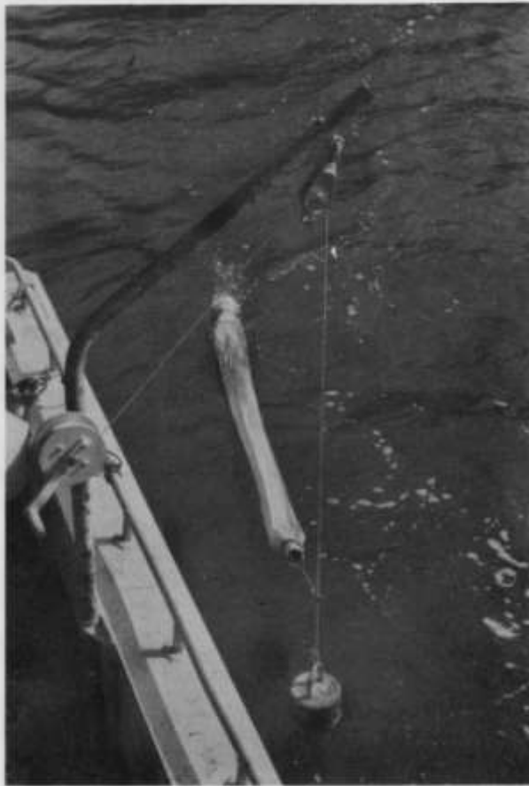
Fig. 27. Plankton net used for transect mussel larvae sampling. The lead weight maintains the net's depth position.
