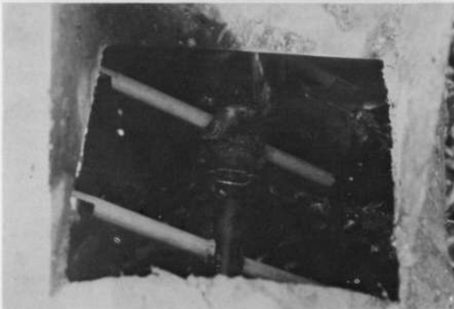
Fig. 75. (Upper) Simple washer and declumper for small lot harvesting. (Lower) Close up of centre revolving shaft.
