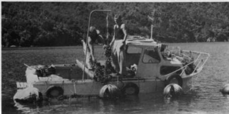
Fig. 65. A welded steel boat used for servicing long lines and harvesting mussels up to one tonne/day.
