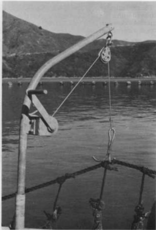
Fig. 66. Simple hand winch used for partially lifting and servicing long lines.
