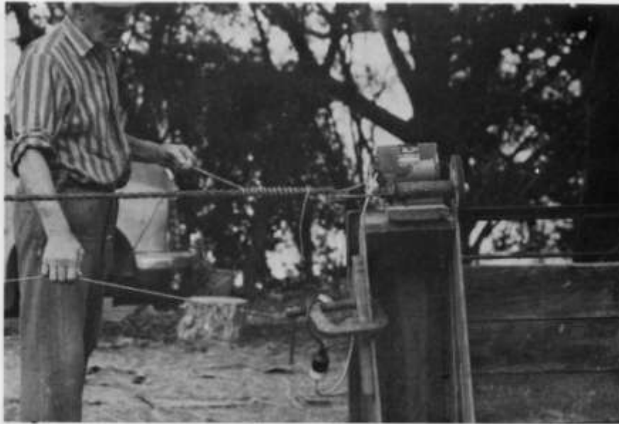
Fig. 62. Wrapping coir on ropes with electric motor. The rope opposite end is held with a ball bearing swivel hook and rubber strap.
