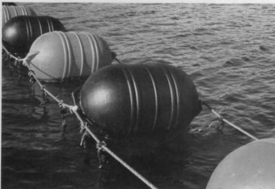
Fig. 48. The long line main lines are usually 18mm polypropylene superfilm. Buoy spacing varies but shown at 2 metres while culture ropes are at .5 metre spacing. (Photo taken of early demonstration long line having alternating black/orange buoys.)
