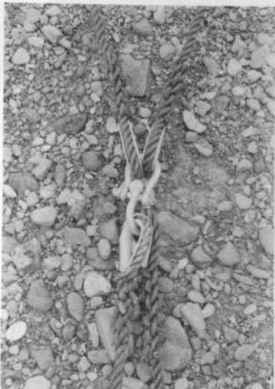
Fig. 50. (Left) Long line bridle extending to two 18mm polypropylene anchor lines, or (Right) to one 24mm polypropylene anchor line.
