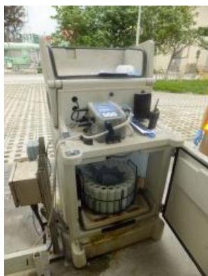
Photo 4-1 Hach Sigma AWRS Sampler
