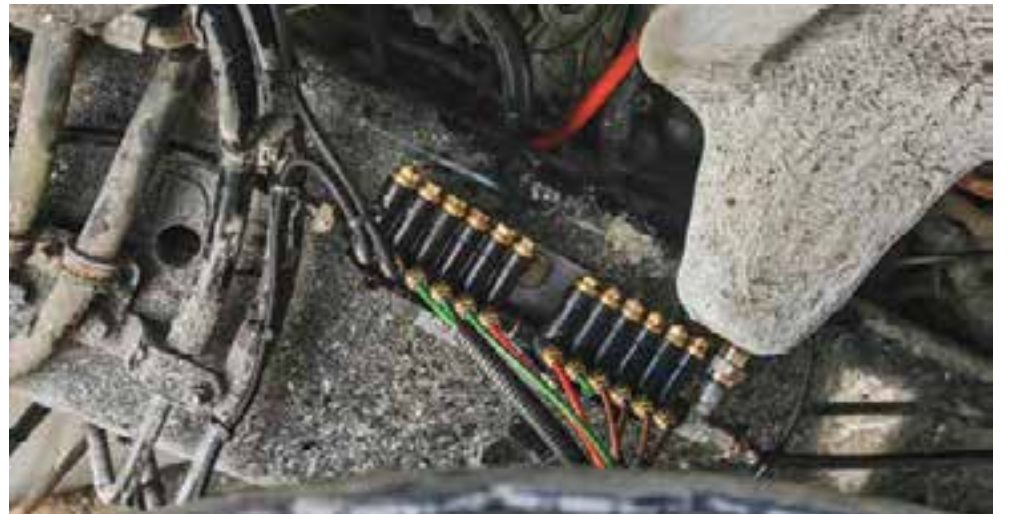
FLO Lubrication System is adaptable to serve a truck's various possible attachments. Hydraulic quick disconnects allow the addition of new lubrication points to the existing system.
