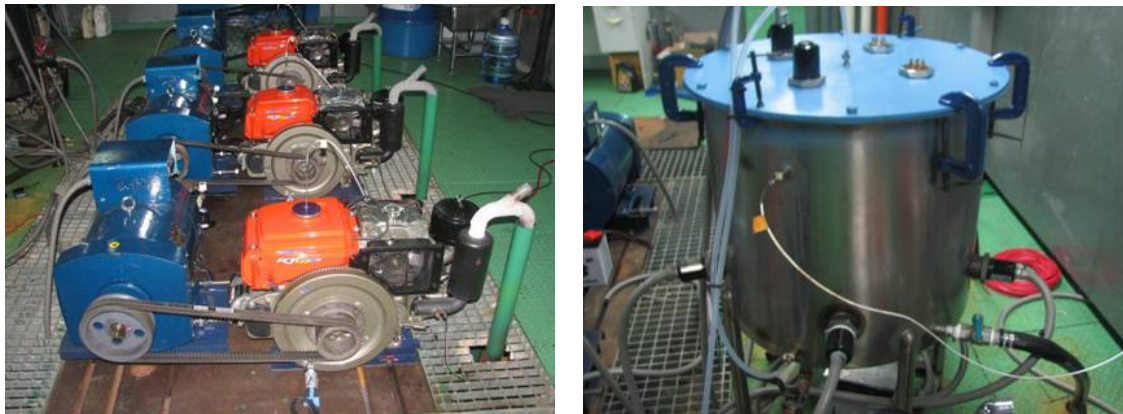
Figure 50 Experimental setup showing (a) Kubota engine coupled with electricity generator and (b) resistance heater coil
