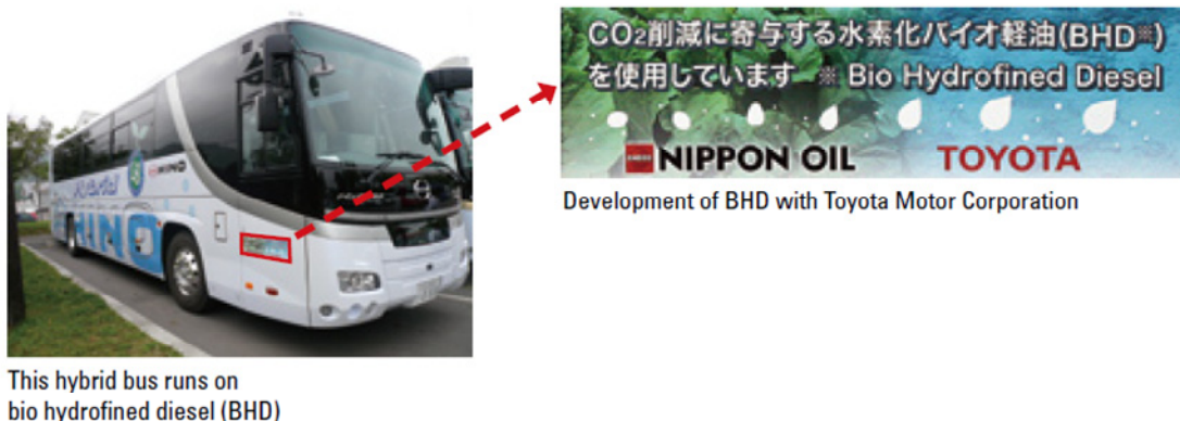
Figure 77 On-road testing of hydrogenated bio-fuels using a hybrid bus
