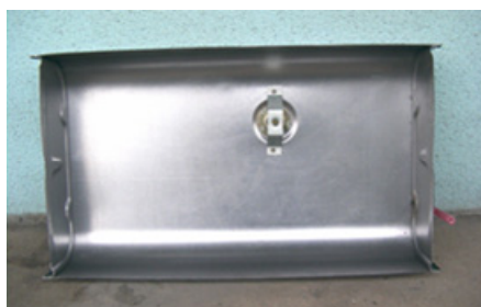
Figure 16 Effects of oxidation stability on fuel tank corrosion
