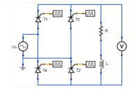
When I<sub>T3</sub> and I<sub>T4</sub> are triggered, commutation occurs from I<sub>T1−3</sub> to I<sub>T2−4</sub>.
