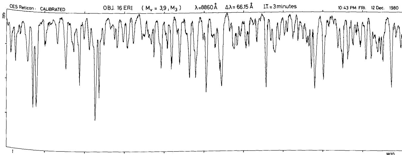
One of the first spectra obtained with the Coudé Echelle Spectrometer and the Coudé Auxiliary Telescope. The star 16 Eri has been observed in the near infrared with a resolution of 90 mA. The total length of the spectrum is 66 Å. The very high signal-to-noise ratio obtained with only 3 minutes integration illustrates the high efficiency of this instrument.
