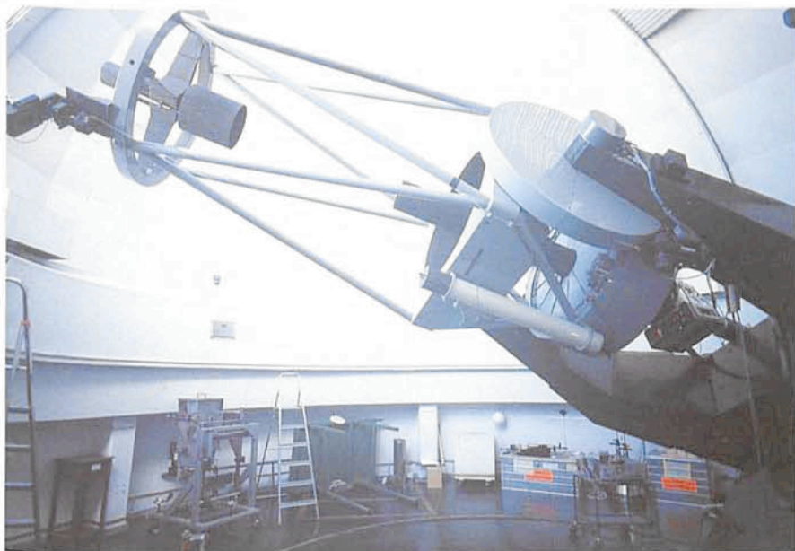
Figure 1: The 1-m telescope with focal reducer in its unusual position to observe Comet Wilson. Two small wide-field photographic cameras are mounted on the front ring.
