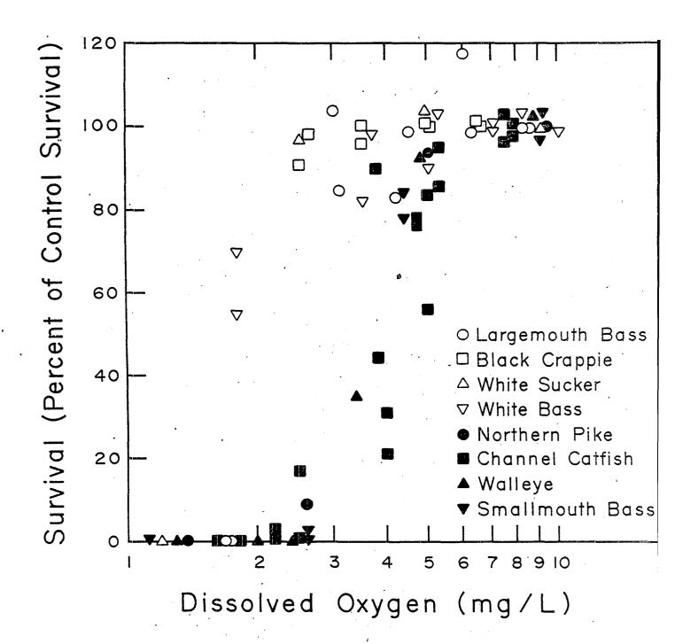
Figure 1. Effect of continuous exposure to various mean dissolved oxygen concentrations on survival of embryonic and larval stages of eight species of nonsalmonid fish. Minima recorded in these tests averaged about 0.3 mg/l below the mean concentrations.
