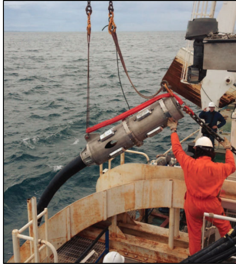
Figure 0-7. Example of subsea connector (MacArtney's GreenLink Inline Termination).
