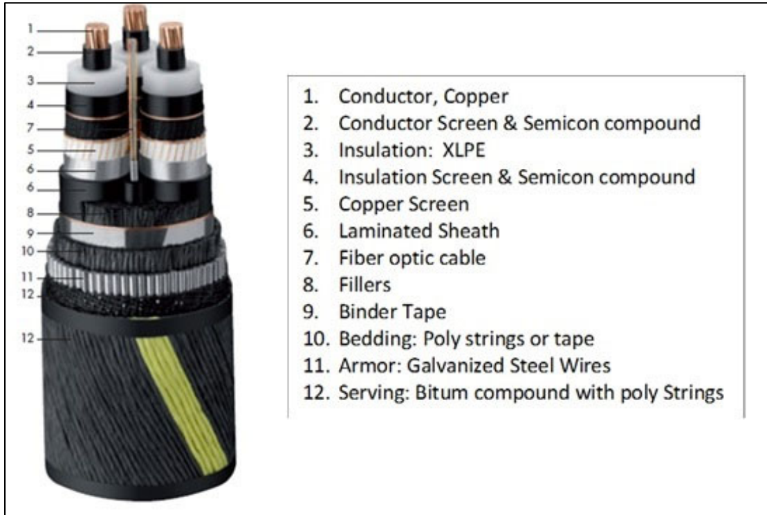
Figure 0-8. Example of medium-voltage subsea cable.
