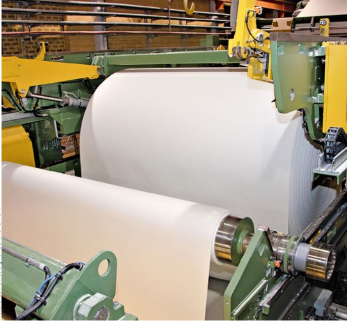
Winder unwinder section with new parent reel feeding and empty spool lifting.
