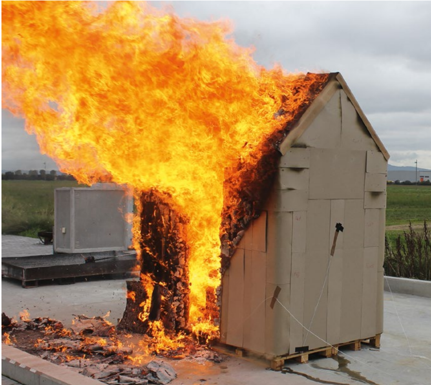
Picture 2: Flammability test with a demonstrator house.
