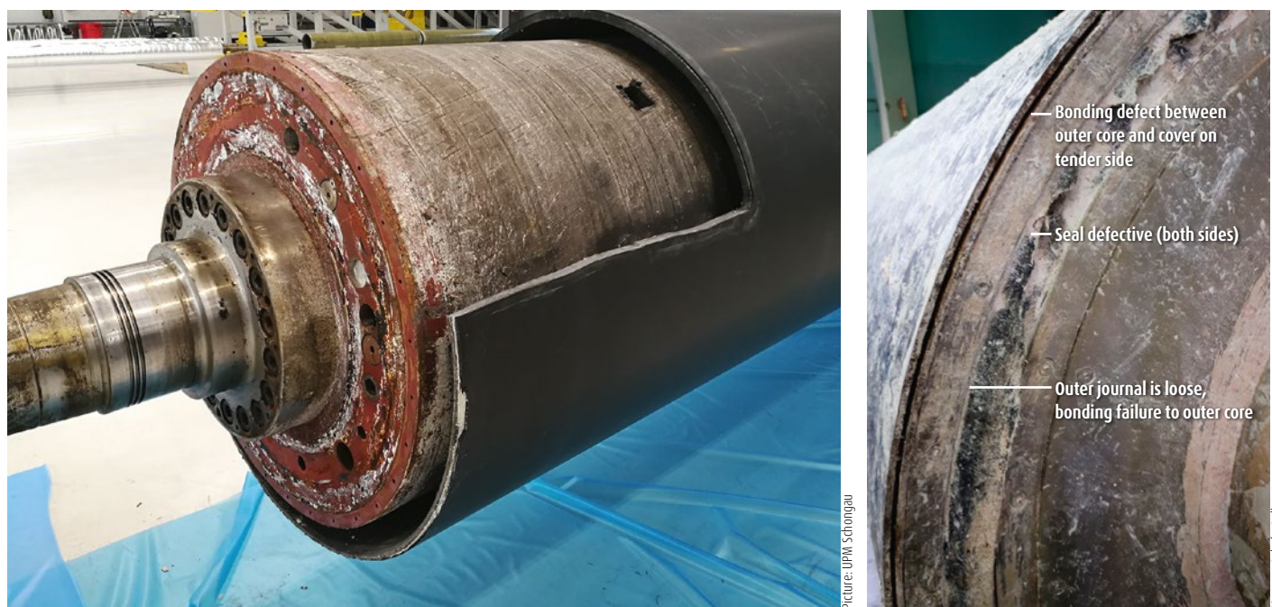
Fig. 1: Previous design shows distinct weak points
