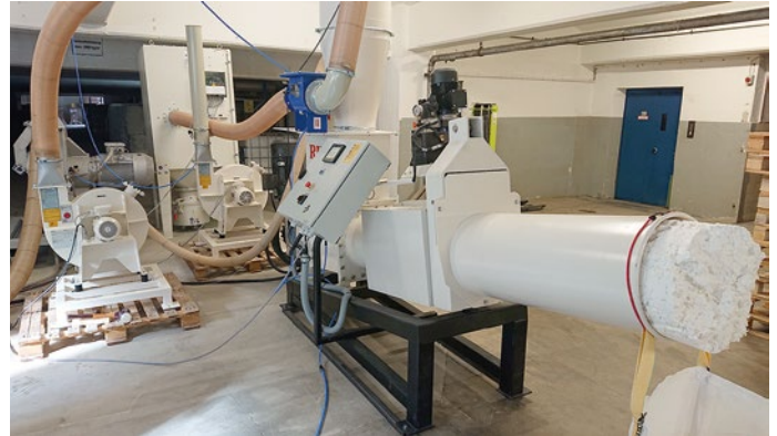
Fig. 4: Compressed dry fibres are successively discharged from the fibre compressor of the mobile dry defibration plant
