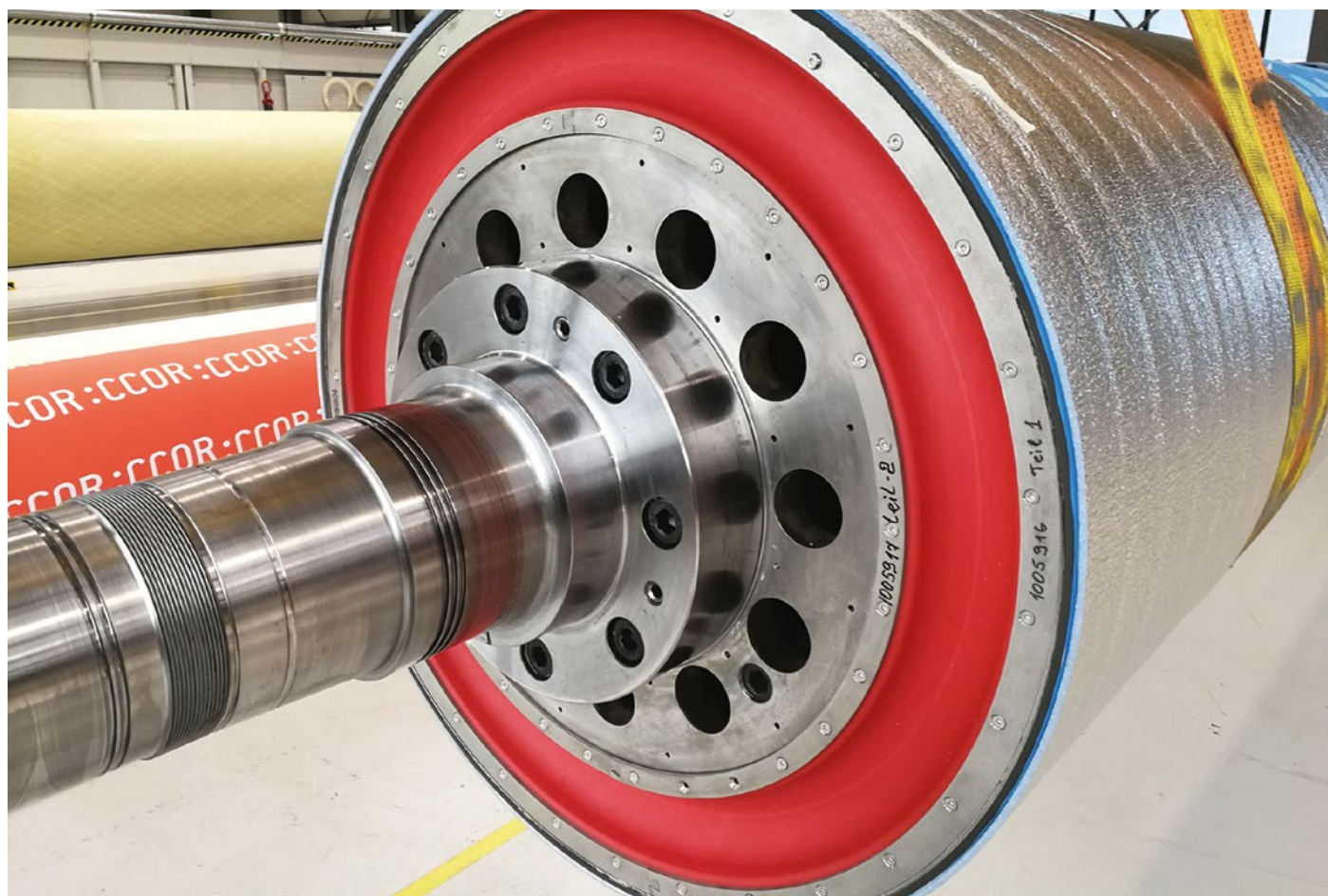
Fig. 4: Double-conical CSR roll with special seal ready for delivery
