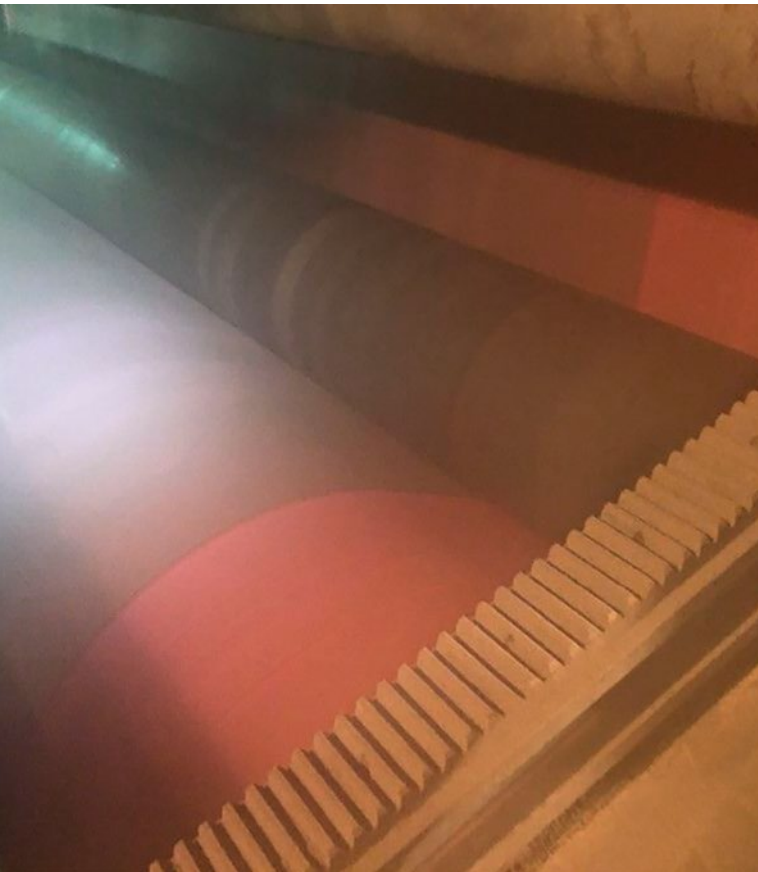
Fig. 7: Cleaning result on roll side of the fabric during the first traversing
