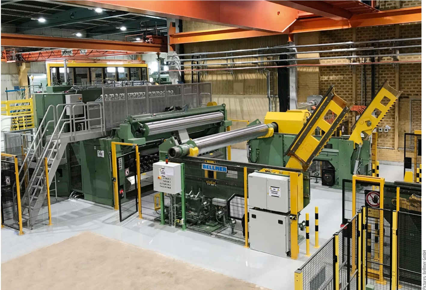
Start-up of the new Bellmer reeling, transporter and winding section.
