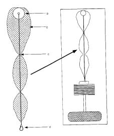
Figure. Mesh collector (left) and modified crevice collector (right). The mesh collector consists of a) 15 cm diameter styrene float; b) nylon trawl mesh bundled and tied to the main float line; c) 8 mm rope connecting snap clip and float; d) snap clip for attaching mesh to the top of a standard crevice collector.
