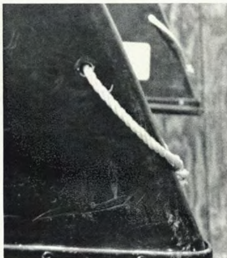
These canoes have holes for endlines. This modification aids lining and makes cartopping easier.
