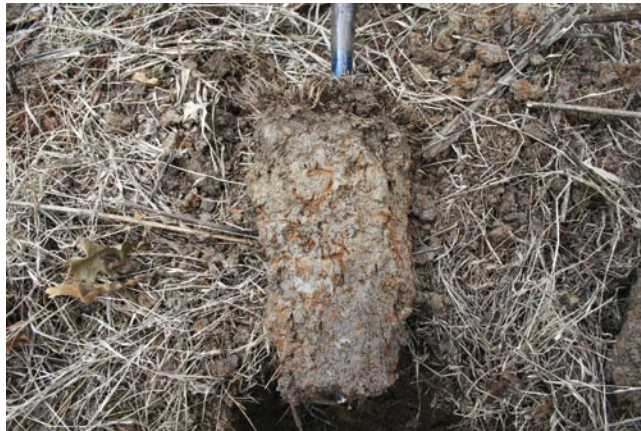
Figure 46.—A depleted matrix with value of 4 or more and chroma of 2 or less and with redox concentrations occurring as soft masses and pore linings.
