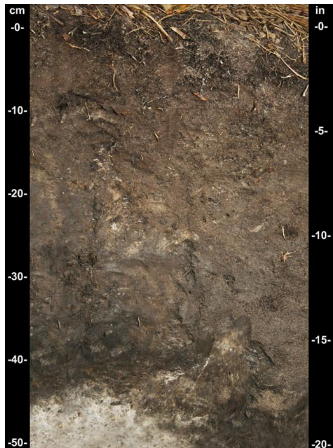
Figure 31.—Indicators F6 (Redox Dark Surface) and F7 (Depleted Dark Surface). A soil that meets the requirements of indicator F7 commonly also meets the requirements of indicator F6. If the dark surface layer has depletions, it most likely also has concentrations.
