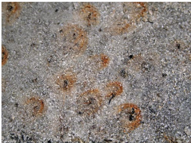
Figure 23.—Indicator S5 (Sandy Redox). A close-up of the layer in figure 22 that has chroma of 2 or less and at least 2 percent redox concentrations.
