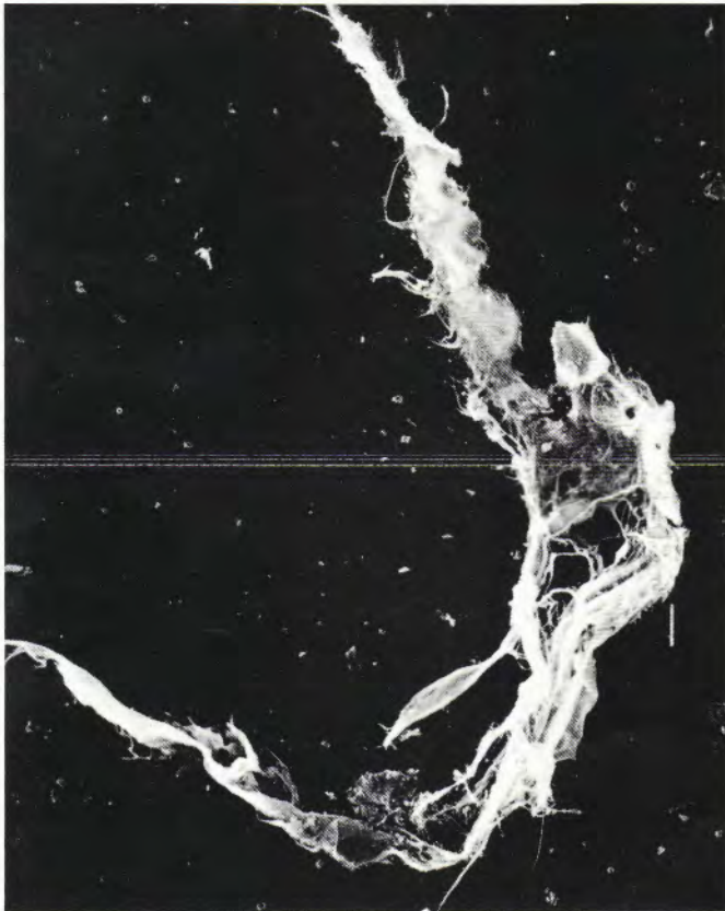
Figure 1. Scanning electron micrograph of rutile "mountain leather." Maximum dimension of aggregate is about 2.1 mm. White bar to right of aggregate represents 100 micrometers.
