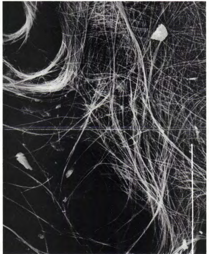
Figure 2. Scanning electron micrograph showing fibrous habit of rutile "mountain leather." Length of field is about 0.1 mm. Small white bar represents 10 micrometers.
