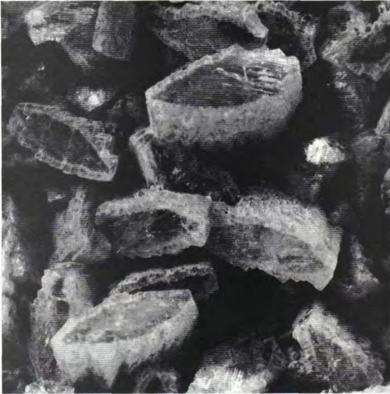
Figure 5. Appearance of a hand-specimen of marsturite overgrowths on rhodonite; Franklin, New Jersey. Long dimension of the crystals is 3–4 mm.
