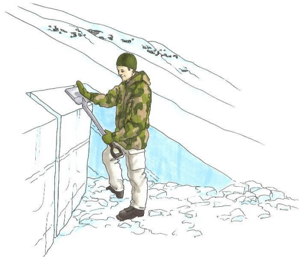
Figure 7.6: Extended compression test (ECT) A 30x90 cm column is loaded with up to 30 'strikes', as for the compression test.
