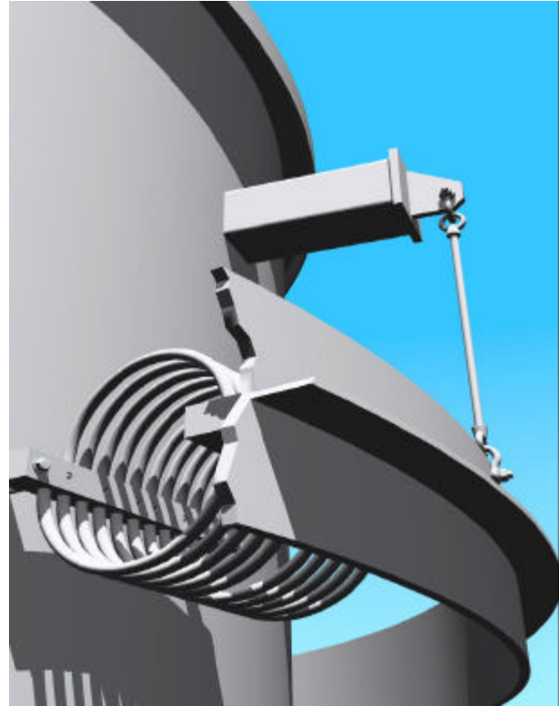
Cutaway Rendering of a Tuned Mass Damper
