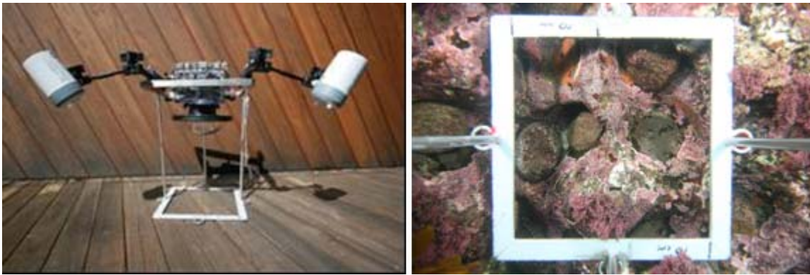
Figure 7. Images of: a) the camera and photoquadrat frame used, b) photoquadrat frame located over fixed markers.
