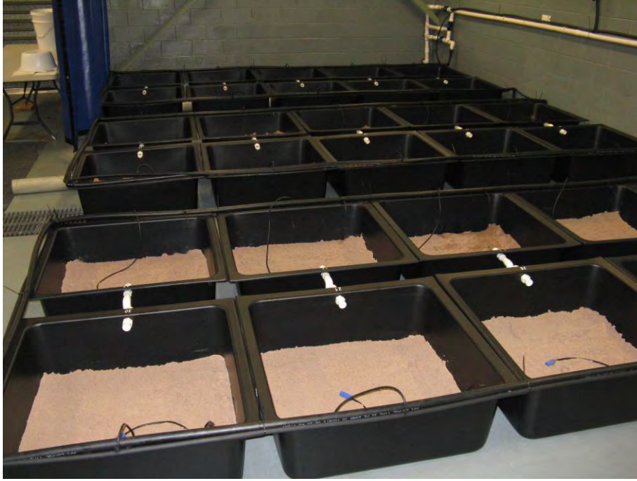
Figure 2.2: Experimental system for Holothuria scabra brood stock maturation trials. Each tank supplied with filtered seawater and aeration. Set up was in a temperature controlled room.
