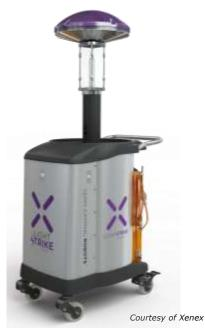
Beyond destroying microorganisms effectively, the highintensity pulsed xenon UV light operates more quickly than other UV technologies. For example, the LightStrike robot runs an average of 5 minutes to deactivate C.diff spores compared to mercury bulbs requiring a 52-minute run time.
