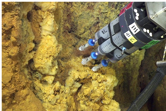
A Bio-Mat sampler allows the scientists to gather just the top layer of the mat at Seamount X, where it is believed all the active microbes live. Photo: NOAA
