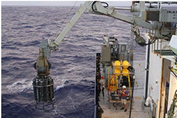
A CTD instrument package is launched over the side of the ship to search for hydrothermal plumes at Ahi Seamount. Photo: NOAA
