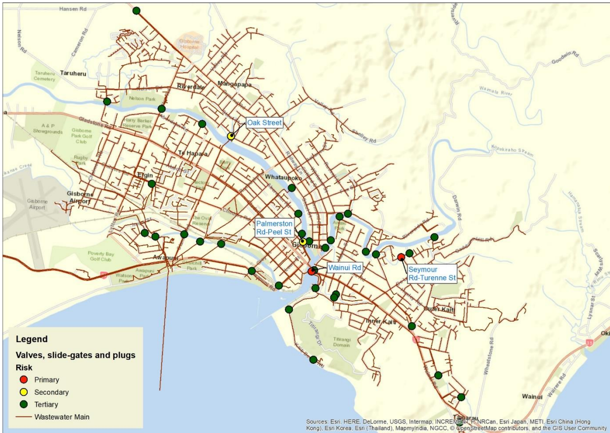
Figure 2-2: Gisborne overflow points controlled by valves, slide gates and plugs. Primary, secondary and tertiary overflow points are shown, with the primary and secondary points labelled.
