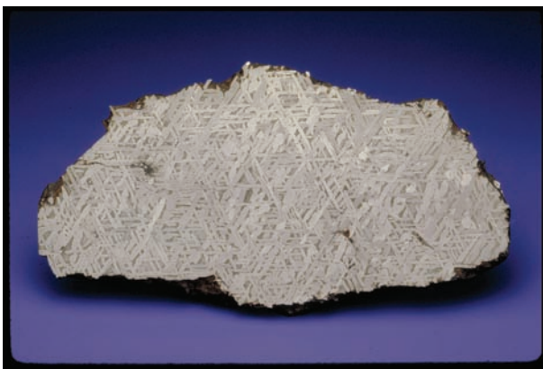
FIGURE 4. The Staunton iron meteorite (USNM 590), ~20 cm in length. This polished and etched slice displays the distinctive Widmanstätten pattern characteristic of many iron meteorites, with plates of low-Ni kamacite (Fe,Ni metal) exsolved from high-Ni taenite at cooling rates of 1–100 °C/Myr. Iron meteorites sample the cores of differentiated asteroids, provide some of our best clues to the chemical nature of our own core, and continue to fall to Earth. Photo courtesy of T. McCoy.
